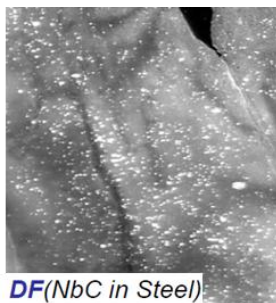
Figure 6.2: shows Dark Field (DF): excludes transmitted electrons. Resolving Power: 1-2nm
